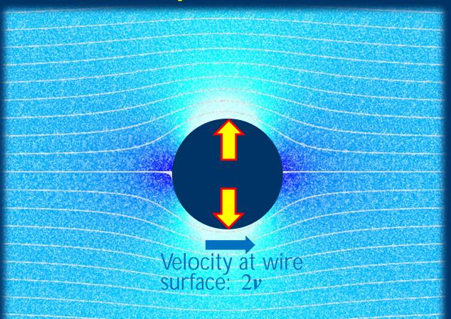
The wire sees the bulk liquid approaching at velocity *v*,
