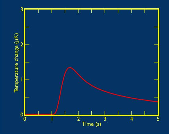
So, just emitting these very few excitations off a very small area of the wire increases the temperature of the whole <sup>3</sup>He liquid volume by ~1.5  $\mu$ K.
