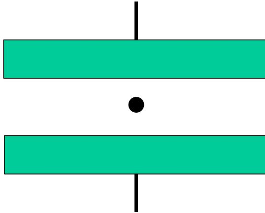
Nb capacitor: spacing 1 mm, diameter 4mm
